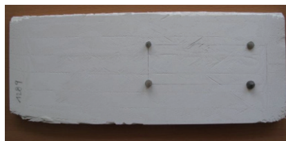
图14 氧化物纤维增强陶瓷基复合材料 Fig.14 Oxide fiber reinforced ceramic composites
